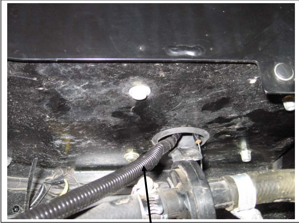
Wire coming from the thermostat to the pressure switch.
