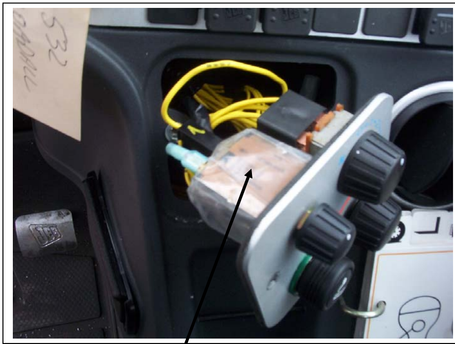
Install thermostat as shown.
