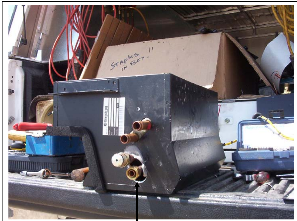
Mark and cut holes in the heater box to accommodate A/C fittings.
